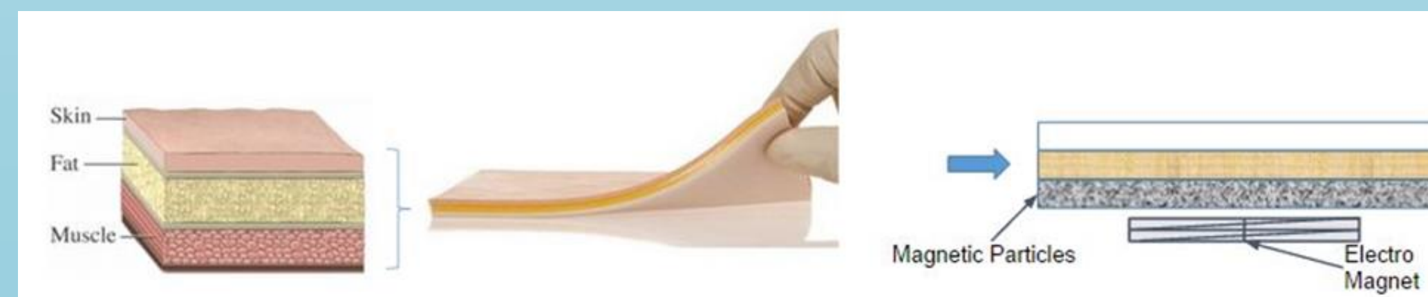
Figure 4: A diagram indicating human skin structure, and the proposed MRE artificial skin model.
