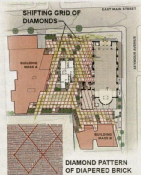
Figure 4 - Site diagram demonstrating how the diamond pattern is incorporated into the site design
