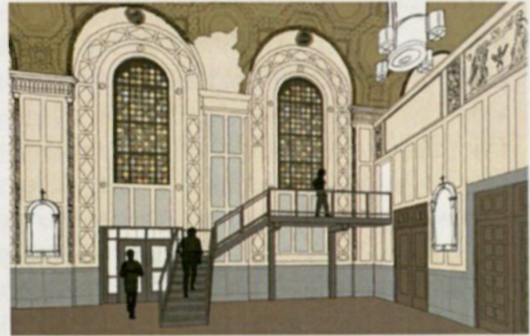
Figure 10 - Rendering of interior showing new stair to mezzanine along with ceiling repair and interior painting strategy.
