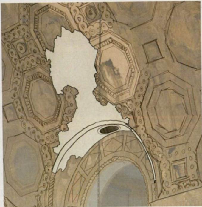
WEST TRANSCRYPT CEILING DAMAGE REPAIR NEW SMOOTH LAYER SET BACK SLIGHTLY FROM HISTORIC PLASTER
