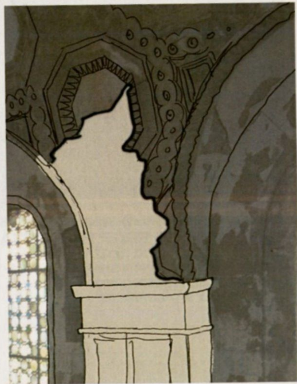
REPLACEMENT FOR DAMAGED PILASTER HEAD NEW SIMPLIFIED COLUMN HEAD TO DIFFERENTIATE NEW ELEMENT TO REPLACE ONE LOST TO TIME
