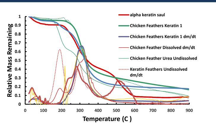
TGA results, above and below, show the varying thermal stabilities of all keratin samples tested. The mass temperature profiles are indicative of the types of polypeptide bonding in the structures.
