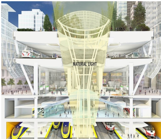
Figure 19: Transbay Transit Center Section
